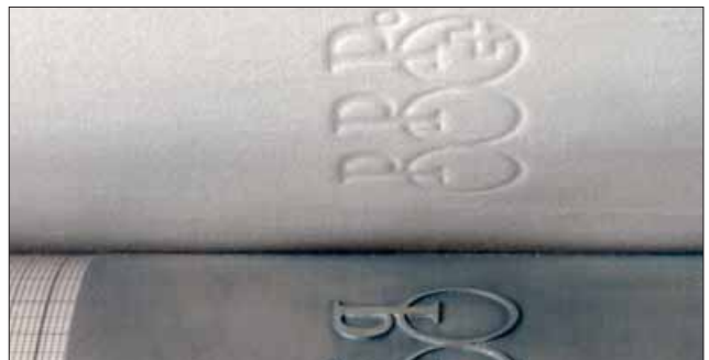
Embossing Dies with Rubber for Scoring
