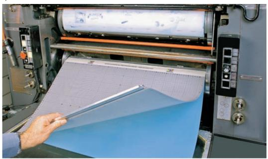
1d Inch the cylinder forward until the rear clamping bar of the base foil can be hooked into the bar holder on the blanket cylinder. For precision installation of the base foil, the bars have to be installed strictly parallel to the cylinder gap.
